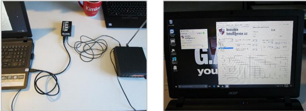
Figure 3.3. G.A.R.D. Final Installation Hardware (left) and Graphical Interface (right)
